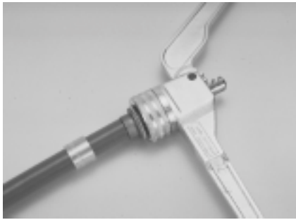
Fig 2.9: Compression sleeve installation steps.
